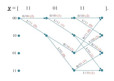
The number in parentheses on each branch is the branch metric, obtained by counting the differences between the encoded bits and the corresponding bits in  $\mathbf{y}$ .
